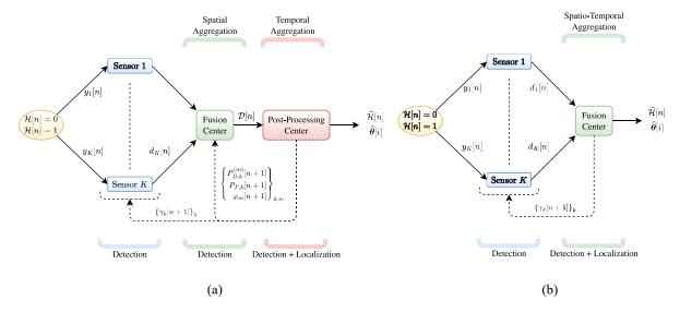
Fig. 2. Proposed WSN architectures (the dotted arrow constitutes the feedback system). (a) Three-layer architecture. (b) Two-layer architecture.
