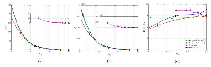
Fig. 5. Performance curves at SNR<sub>m,k</sub> = 0 dB  $\forall m, k$ . (a)  $P_{10}$  versus ADD. (b)  $P_{10}$  versus  $P_{1}$ . (c)  $P_{10}$  versus RMSE.
