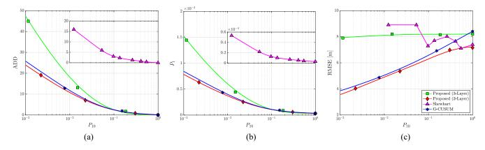
Fig. 7. Performance curves at SNR<sub>m,k</sub> = 10 dB  $\forall m,k$ . (a)  $P_{10}$  versus ADD. (b)  $P_{10}$  versus  $P_{1}$ . (c)  $P_{10}$  versus RMSE.
