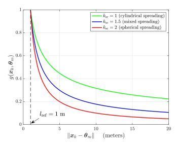
Fig. 3. Attenuation function versus distance between sensor and faulty item.
