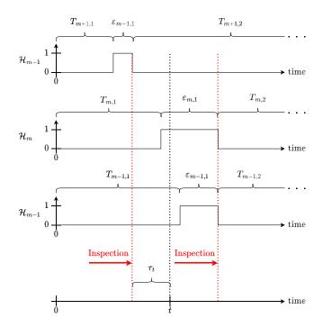
Fig. 1. Failure model (excluding inspection and maintenance durations).
